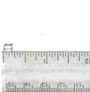
(Ruler Shown to Scale) 3/16" Ignition Probe Gap
