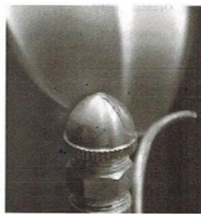
FIGURE 1 Probe Positioned within Flame/Flame Boundry
